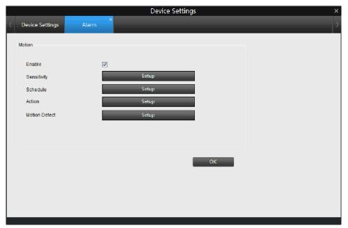
Enable: Turn on motion detection on a specific channel. Each channel can be configured independently.
