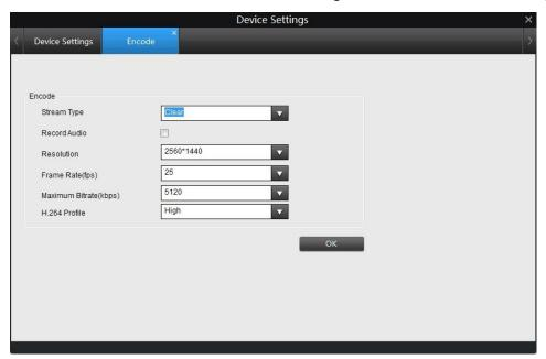
Stream Type: Edit the parameters for the main stream or the sub-stream.
