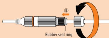
5 Push the rubber seal ring into the waterproof connector and screw the top cover and lock it into position firmly to finish installation
